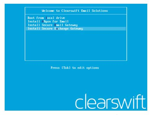
Use the arrow keys or keyboard shortcuts to select Install Secure Exchange Gateway from the menu. Press the Enter key to select the installation.
